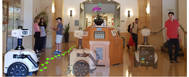
Fig. 1: Navigation scenario. The (solid) robot needs to reach the back of the foyer. The global planner provides an optimal solution (light green) based on a static environment map. Our navigation approach re-plans locally to adapt to the dynamic environment and control the robot towards the goal (translucent robots).
