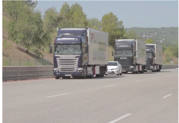
Fig. 1. A human-driven car has cut in between two trucks in the platoon. Such interference may happen if the human is subject to danger in its own lane (e.g., blocked lane by road work), but should in non-critical situations be discouraged due to performance degradation of the platoon.
