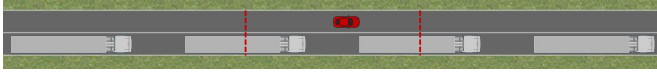
Fig. 2. The four semi-autonomous trucks and the human-driven car on the highway. The interacting truck is currently truck 3 since the car is between truck 2 and 3 (dashed red lines).
